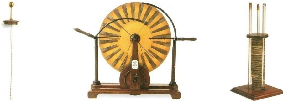
Figure 17: Early electricity producing devices: Lid and chain from a late 19 th century Leyden jar, Wilmshurst machine (1882) for making electric charge, Voltaic pile (1800). 48
