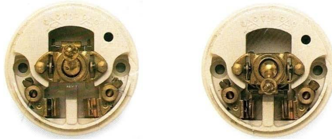
Figure 20: An early ceramic electrical switch. “This early electric switch has the metal components in a ceramic body. Two metal arms are sprung so they flick quickly from one position to another. When the switch is turned on, the arms slot into U-shaped springy contacts, so completing the electric circuit. This must happen fast, and the contacts must be good, or the electricity could spark across any gaps and cause damage.” 53
