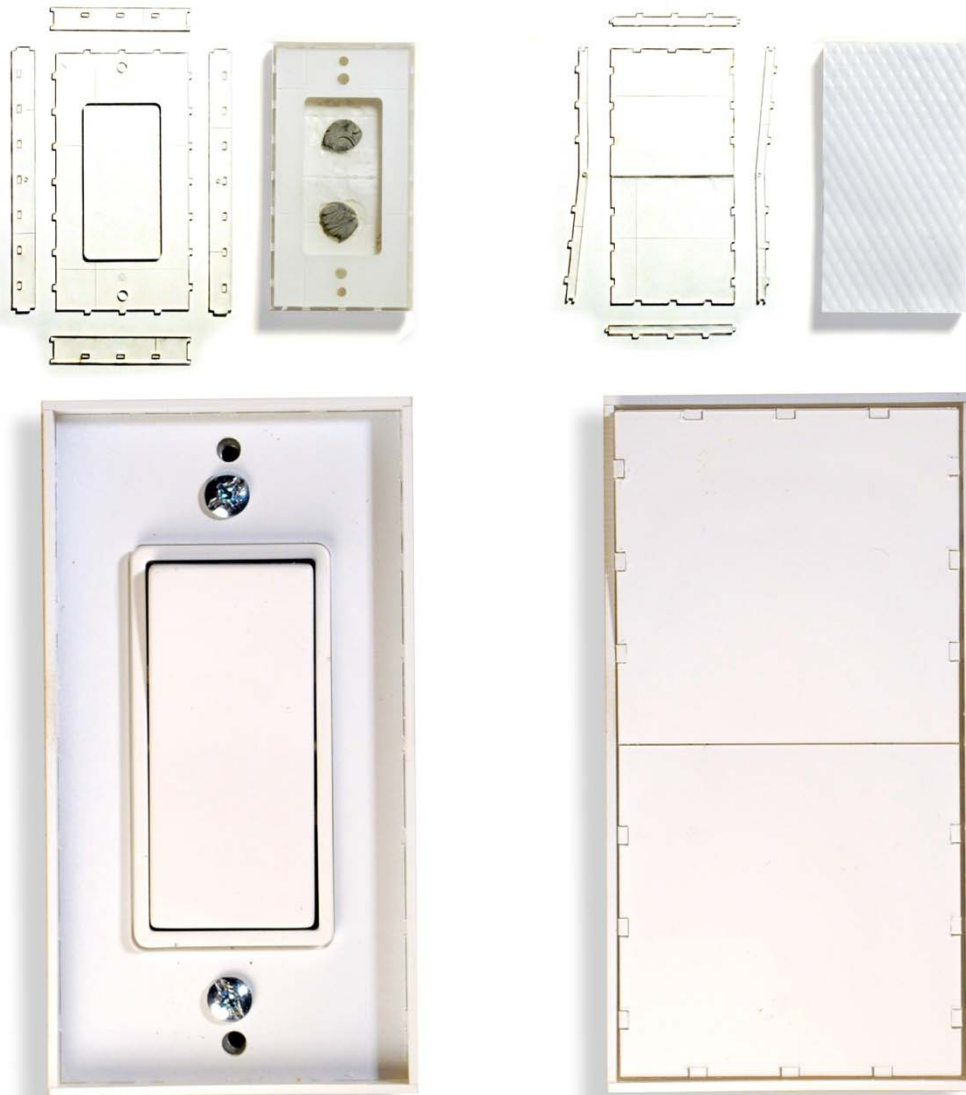
Figure 48: Top- Acrylic pieces cut and assembled to form the secondary safety faceplate and the primary switch plate for this device; Bottom left- Secondary safety faceplate installed over a decorator switch; Bottom right- Primary switch plate snapped in place over the decorator switch and secondary safety faceplate. 109
